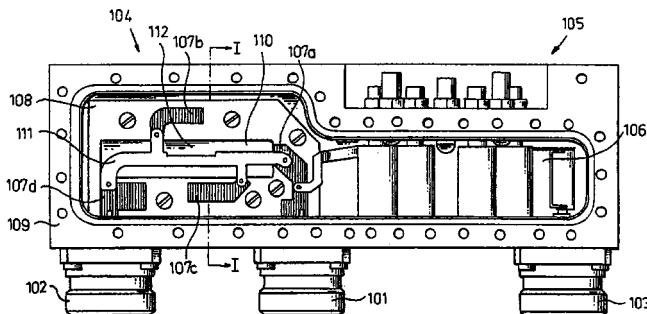
**Dielectric Filter, Dielectric Duplexer, and Communication Apparatus**
